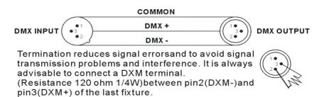
Connect the fixture together in a "daisy chain" by XLR plug cable from the output of the fixture to the input of the next fixture. The cable cannot be branched or split to a "Y" cable. Inadequate or damaged cables, soldered joints or corroded connectors can easily distort the signal and shut down the system.
