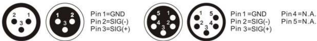
5.1.3 The termination is prepared by soldering a 120Ω resistor between pins 2 and 3.
